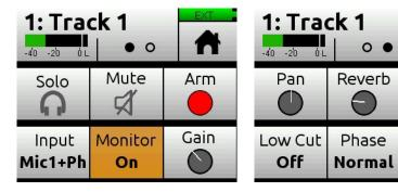
Each Channel screen provides two pages of settings—indicated by Dots icon. Tap the Dots icon to switch pages.
