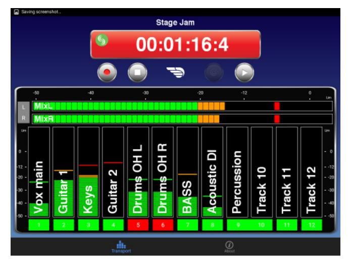
① Custom naming and arming of tracks may be done in Transport view (shown above) on large screen mobile devices, like tablets, or in Track view on smaller screen mobile devices, like smartphones.
