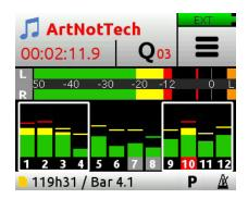
Track labels, each bearing the track number, appear along the bottom of the meter view and will change color based on routing and transport status.
