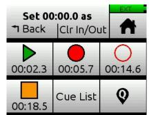
① It is not possible to place an In point after an Out point. It is also not possible to have more than one In or Out point of each type (Play or Record).
