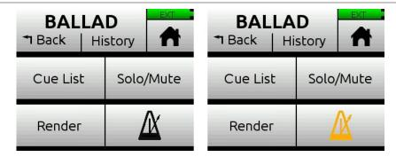
(1) The Metronome button will be disabled (appearing grayed out but with an orange icon) whenever Click is assigned as a track's input source.
