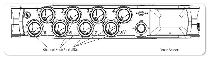
The LEDs around any of the bottom four knobs will also pulse orange if, upon changing track banks, the knob's rotational position is not aligned with its fader value; this pulsing stops once position and value are realigned. For more information, see *Track Bank Selector*.
