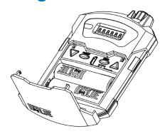
IFBR1C functions with two (2) AA batteries (+1.5 VDC each); alkaline, lithium, or NiMH rechargeables (supplied). Pinch the buttons on each side of the battery door, and pull the door toward you to open. Install the batteries according to the polarity diagram. Select either "primary" (non-rechargable) or "NiMH" (rechargeable) via the slide switch next to the USB connector. Press the battery door closed until you hear the retaining clasps snap.
