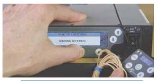
NOTE: You must position the transmitter's IR port directly in front of the DSQD IR port, as closely as possible, to guarantee a successful sync. A message will appear on the DSQD if the sync was successful or failed.
