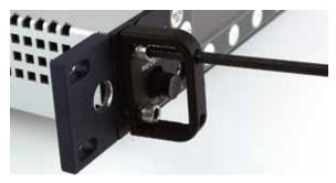
5. If antennas will NOT be mounted on the front panel of the receivers, install the hole cap (Part #35959) by aligning the flat on the cap with the flat on the opening.
