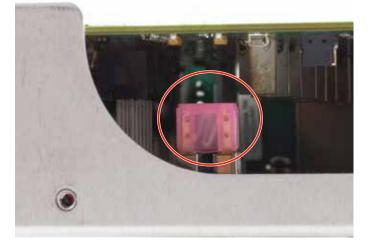
This is a standard 4A, 32VDC mini blade (automotive type) fuse. You can obtain one from any automotive or electrical supply shop, or order one from us (part #21941). Replace if necessary.
