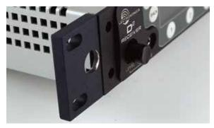
4. Insert two (2) cap screws (Part #28885) through the rack handle (Part #27082) holes and install the rack handle onto the flange bracket through the holes in the unit's front panel. Firmly tighten the cap screws using the hex key (Allen wrench) as shown.
