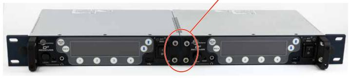
7. Remove the four cap screws from the adjacent rear panels, and then use them to attach the rear tie bracket. Do not tighten the screws completely.
