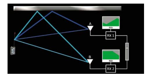
• **Frequency:** Again, the receiver channels are paired. In this mode, each channel is set to a different frequency. The DSQD automatically uses whichever receiver's RF signal quality is better. The use of separate frequencies helps minimize dropouts caused by multi-path phenomenon. This technique uses both switched and vector diversity for maximum effectiveness.
