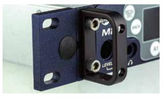
6. Install the Front Tie Bracket (Part #25991) into the open slot in the right side of the M2T Chassis Cover Panel with the protruding nuts facing rearward, affix with two (2) Cap Screws (Part #28885) provided and firmly tighten with the Hex Wrench. See next page.
