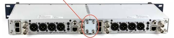
8. After front and rear tie brackets are installed, place the receivers on a flat surface so the that the front panels are even with each other. Hold the receivers in place and tighten all cap screws on the front and rear brackets.
