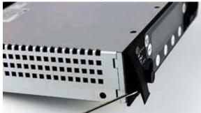
2. Remove the breakaway tabs on both sides of the chassis side panels. Use a flat blade screwdriver to pry the tabs outward and snap them off of the chassis.
