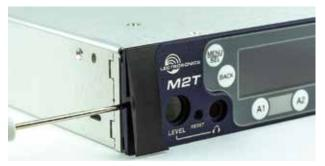
2. Remove the breakaway tabs on both sides of the Chassis Cover Panel. This requires the use of a flat-blade screwdriver inserted into the slots and levering the tabs away on each side of the unit.
