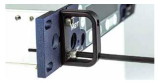
5. Unless also installing a Front Mounted Antenna, insert the Hole Plug (Part #35959) into the open antenna hole in the Flange Bracket by aligning the flat sides of the plug with those of the bracket hole and pushing into place until flush.
