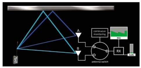
• **Vector:** In this mode, two receiver channels can be "paired" as one receiver. Either Channels 1 and 2 or channels 3 and 4 can be combined into a pair. One receiver in a pair is fixed on Antenna A and the other receiver in a pair is fixed on Antenna B. The DSQD automatically and optimally combines the intermediate frequency signals.
