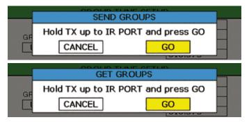
When a tuning group is assigned, the frequency control is limited to the frequencies contained in the tuning group. It also limits the available frequencies in the frequency coordination process.
