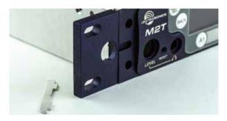
4. Insert two (2) Cap Screws (Part #28885) through the Rack Handle (Part #27082) holes and install the Rack Handle onto the Flange Bracket through the holes in the unit's front panel. Firmly tighten the Cap Screws using the long leg of the Hex Wrench as shown.
